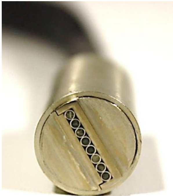
Figure 5.1: Patient end of CYRIL 1 with 4 detector fibres held in a probe holder and two source fibre heads. Taken from [111].
