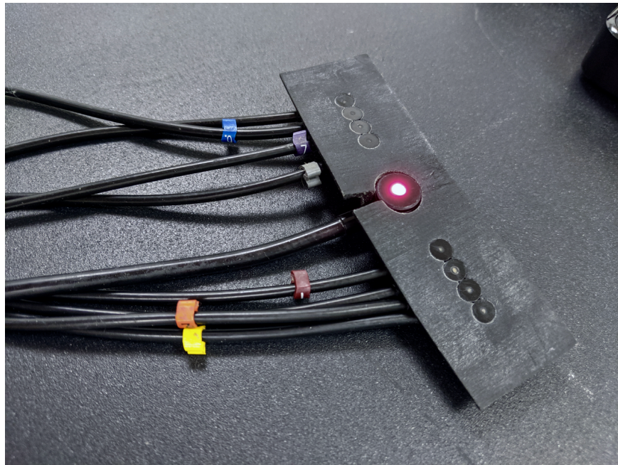
Figure 5.8: CYRIL 2 probe holder with widened sides. The light source is in the middle, with four detectors on each side.
