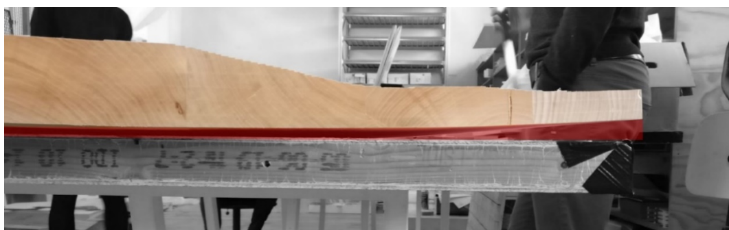
Figure 5.7 Warping of the timber model after the robotic milling operation due to changes in the internal stresses of the grain.
