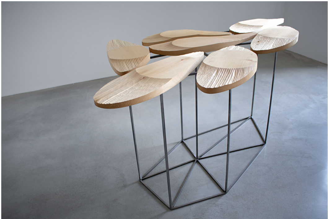
Figure 5.23 The demonstrator is composed of a series of robotically-carved wooden platforms to exhibit art objects.
