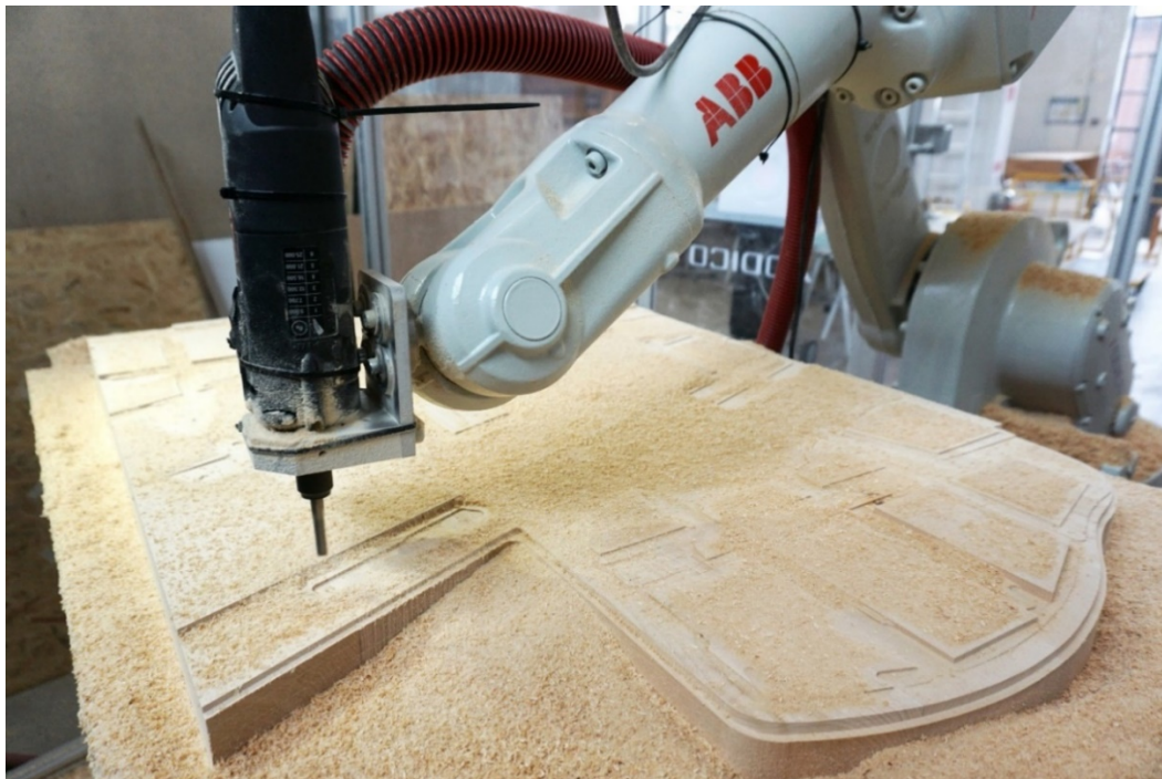
Figure 5.4 Robotic milling of one of the timber modules of the BIG U model.
