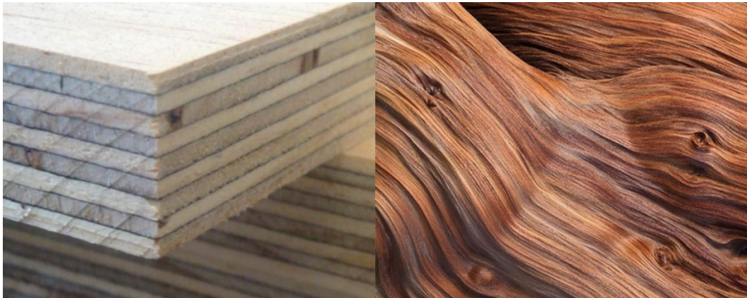
Figure 2.5 Comparison between plywood and natural timber - Sources: plywoodmaster.com (left), Lee Rentz (right).
