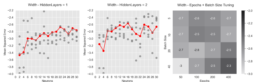
Figure 4.28 Depth feature prediction: optimisation of the ANN topology ( i.e. the number of hidden layers and neurons) and hyperparameters ( i.e. epochs and batch size).
