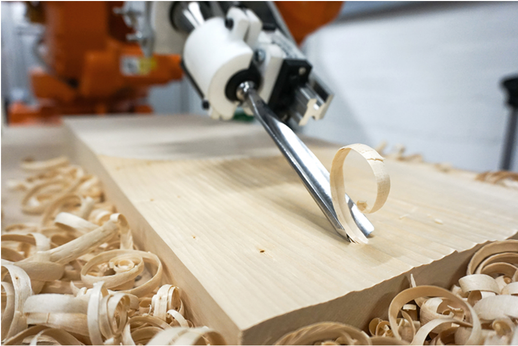
Figure 5.33 Robotic carving process of one of the demonstrator's components.
