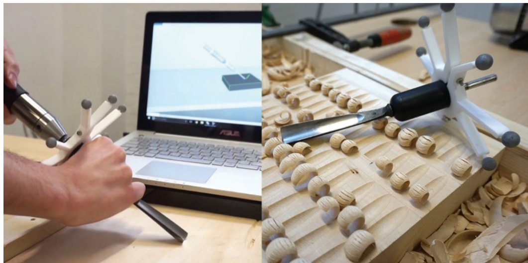
Figure 3.7 Custom tracking markers are applied to the carving tools to reconstruct in real-time their position and orientation in the digital recording environment.
