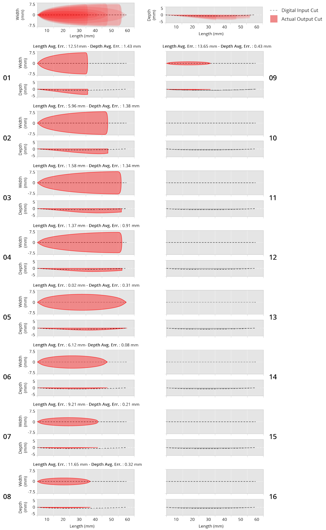
Figure 4.39 Comparison between the input geometry (dashed black line) and the carved one (red). For each operation, top and side views are provided together with the deviation error.
