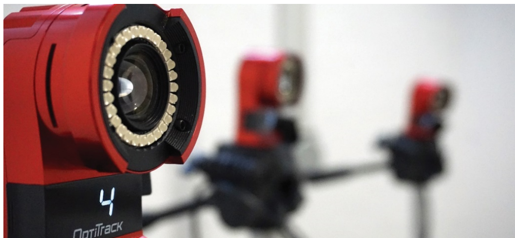
Figure 3.5 Motion capture cameras used in the Recording stage to track the tools and reconstruct the carving operation.
