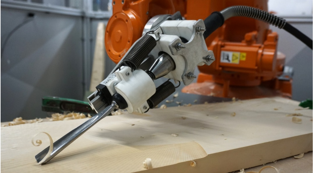
Figure 3.4 Robotic Carving Effector.
