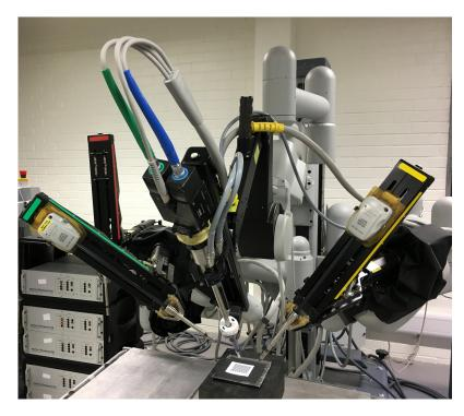
Figure 3.14: Experimental setup for capturing data from the da Vinci Standard.
