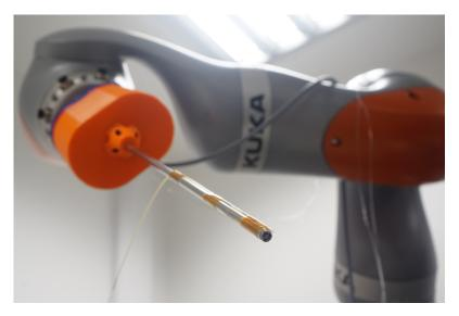
Figure 3.5: Experimental setup for capturing data. The specially designed scope with the NanEye stereo camera is mounted on the flange of the KUKA arm. The scope is 420 mms in length [112].
