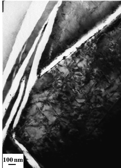
Figure 2. TEM micrograph detailing dislocation debris the microstructure obtained at 250°C.
