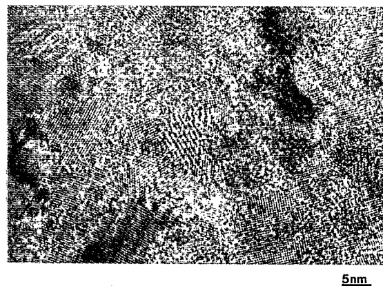
FIG. 8. Typical HREM image of \text{Sb}_{0.71}\text{Ge}_{0.29} film after crystallization, showing the random orientation of the crystalline grains.
