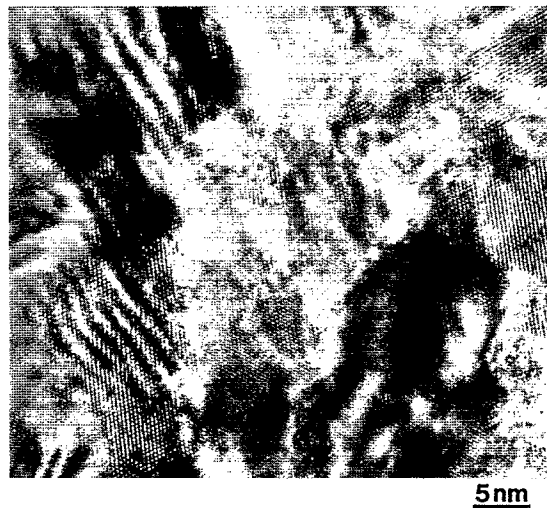
FIG. 5. Typical HREM image showing crystals within a radial grain of a fully crystallized \text{Sb}_{0.89}\text{Ge}_{0.11} film after annealing at 200\text{ }^\circ\text{C} .
