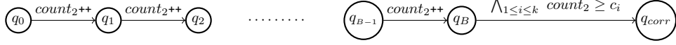
■ Figure 4 Second gadget, which sets up the value of count_2 to be exactly B .
