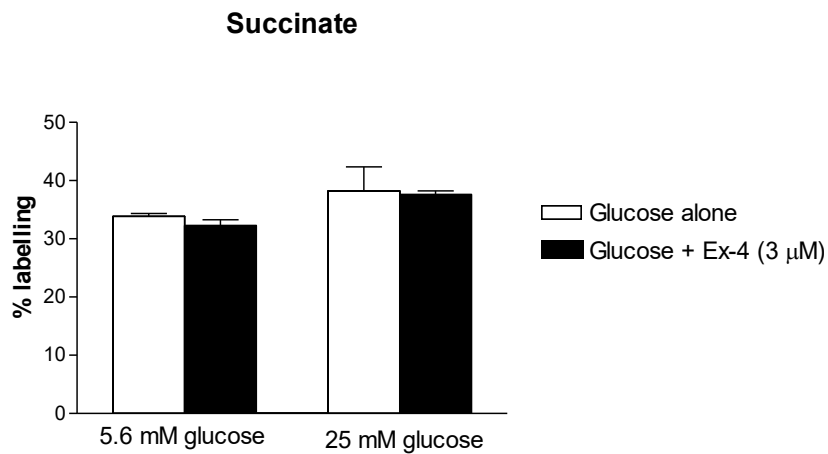
Figure 5.16. 13 C labelling for succinate. Labelling was calculated from the mass isotopomer distributions (MIDs) detected by the GC-MS.
