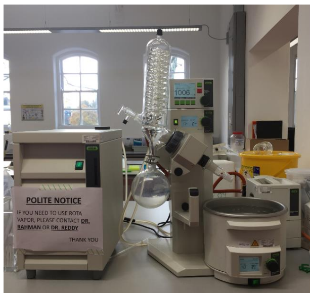
Figure 6.2: Rotary evaporator (Rotavapor®, R-215 by BUCHI) system for solvent evaporation.
