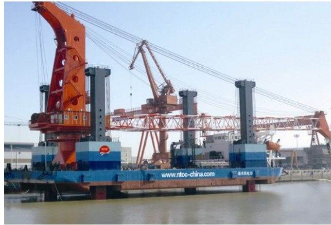
Figure 1: Jack-up wind turbine installation platform (Nantong City, China)
