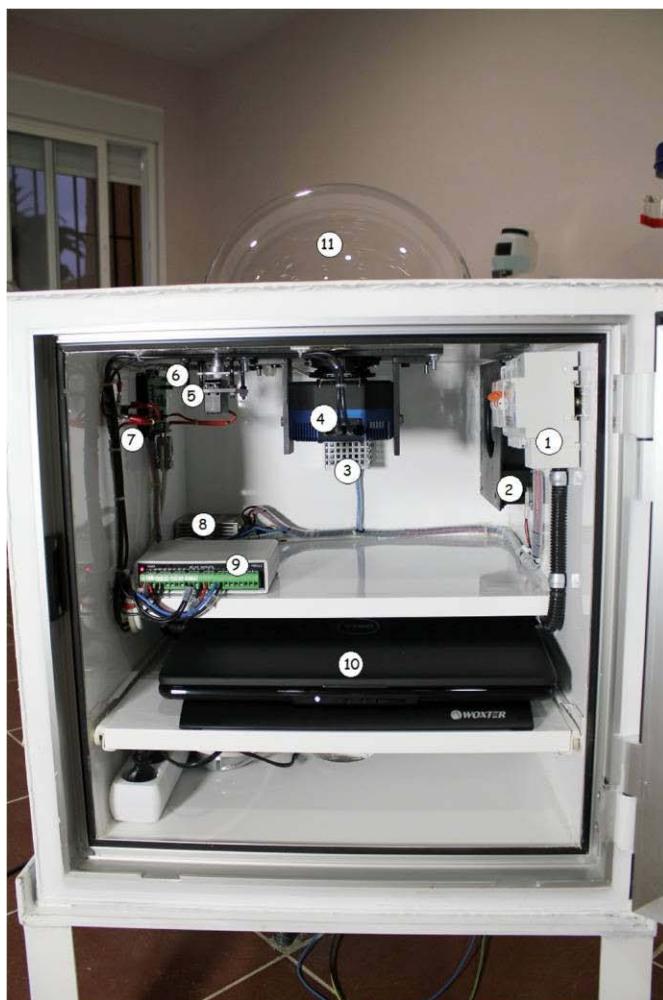
FIG. 2.—Internal view of the system: (1) Ground fault and electrical breakers. (2) Main fan. (3) Antihumidity system. (4) CCD head with filter wheel. (5) Servomotor of the solar shutter. (6) Servomotor controller. (7) Thermostats. (8) Main stabilized power supply. (9) PIC I/O controller. (10) Computer. (11) Acrylic dome. See the electronic edition of the PASP for a color version of this figure.
