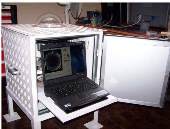
FIG. 1.—External view of an ASTMON unit. The internal components are protected by a weatherproof housing, so the instrument can be installed outdoors. See the electronic edition of the PASP for a color version of this figure.
