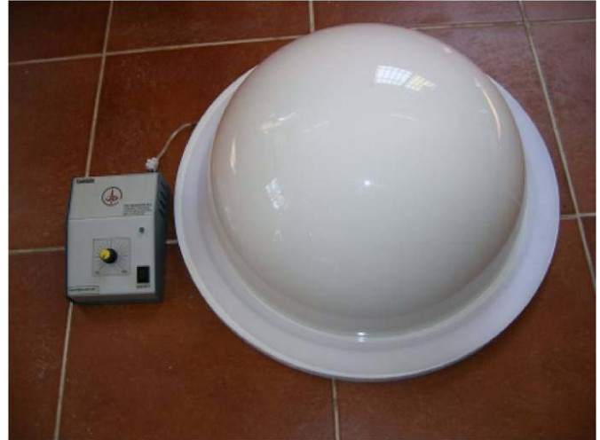
FIG. 5.—Photograph of DomeLight. This device has been developed to uniformly illuminate any wide-field camera. See the electronic edition of the PASP for a color version of this figure.
