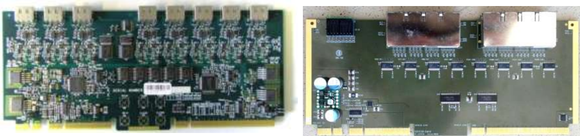
Figure 5. The CERN ADC adapter card (left) and the NEXT LVDS card (right).
