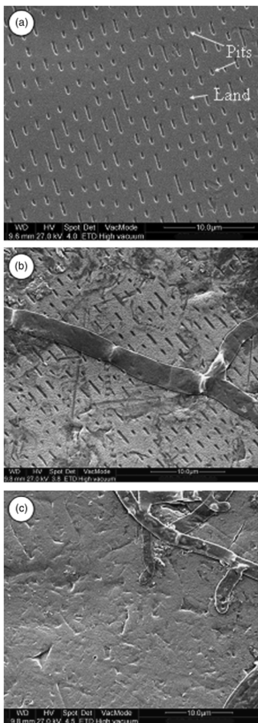
Fig. 2. SEM images of the Geotrichum -like fungus growing on grooved polycarbonate CD fragments and progressive deterioration of pits and lands structures. (a) Control. (b) Fungal hyphae and pits and lands after 1 month of incubation. (c) Disappearance of these structures after 2 months of incubation.
