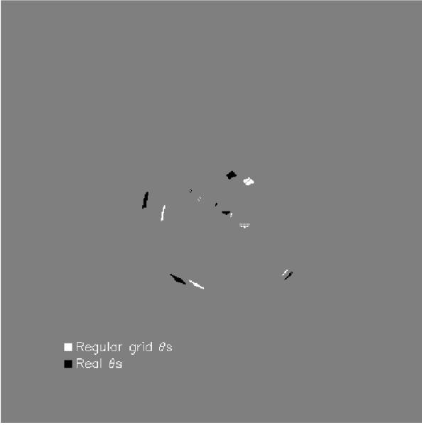
Fig. 2. Simulated observed arcs (black) versus predicted ones from the optimal solution (white). The difference between the two sets of \theta positions is representative of the error expected when recovering the solution.
