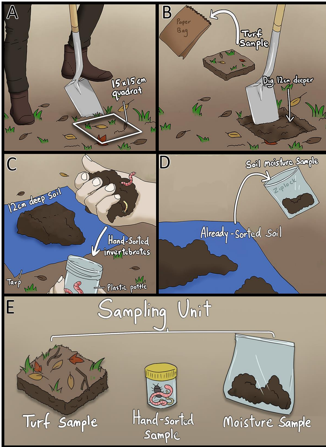
Figure 3.1. Drawings visualizing the protocol for collecting a sampling unit in the field. A) Spade was used to cut into the ground around a 15x15cm quadrat. B) The upper surface of the cut ground (turf sample) was removed and stored in a paper bag. The soil in the remaining hole was dug down to 12cm. C) The soil to 12cm depth was placed on a tarp, then hand-sorted for invertebrates which were placed live into a plastic pottle (hand-sorted sample). D) Approximately 250ml of the remaining soil that was previously hand-sorted was stored into a Ziplock plastic bag for soil moisture analyses (moisture sample). E) The three types of samples collected per 'sampling unit'.
