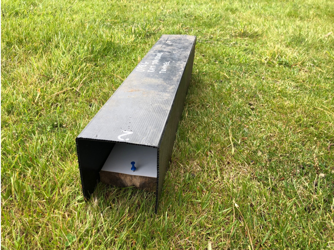
Figure 2.9: Tracking tunnel supplied by the OPBG, with ink tracking card attached to wooden base. Peanut butter used as bait was smeared on both ends of the tunnel.
