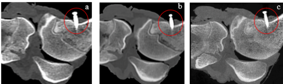
Figure 4.13: Sheep knee with titanium screw (a) single energy CT (b) dual energy CT (c) MARS spectral photon counting CT (75-118 keV). In spectral CT images the soft tissue as well as the trabecular structures in the vicinity of the screw can be clearly visualised.
