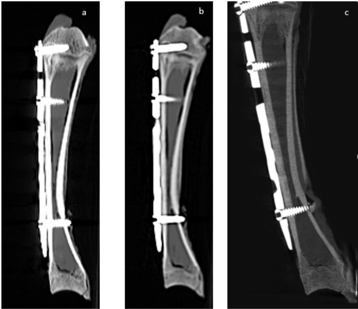
Figure 4.11: Sheep clavicle with titanium plate and multiple screws (a) single energy CT (b) dual energy CT (c) MARS spectral CT (75-118 keV). The photon counting spectral CT images displays how well the grooves of the screw is integrated with the bone adjacent to it.
