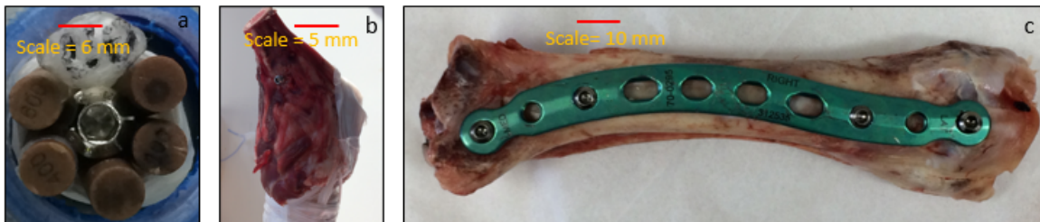
Figure 4.1: Calibration phantom and biological samples (a) A quality assurance (QA) cylindrical phantom containing lipid, water and different known concentrations of HA (104.3, 211.7, 404.3, 604.3 mg/cm 3 ) placed at the vicinity of the screw to assess impact of artefact on concentrations of the known HA rods. (b) sheep knee with titanium screw for quantitative evaluation of bone density and morphology (c) sheep clavicle with titanium plate and multiple screws for qualitative evaluation of streak artefacts at the bone-metal interface.
