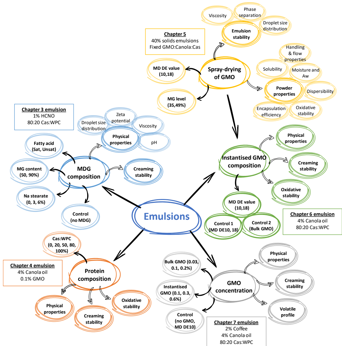
Figure 8.1 Schematic overview of the experimental study design. MDG: Mono- and diglycerides, Sat: Saturated, Unsat: Unsaturated, MG: Monoglyceride, Na stearate: Sodium stearate, Cas: Sodium caseinate, WPC: Whey protein concentrate, MD: Maltodextrin, DE: Dextrose equivalent, GMO: Glycerol monooleate
