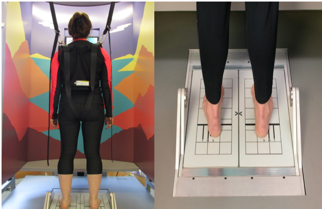
Figure 3.3 Set-up and position of the participant on the EquiTest® balance system machine- the safety harness (left) and foot placement (right) on the force plate ( with signed agreement for talent release-Appendix K ).
