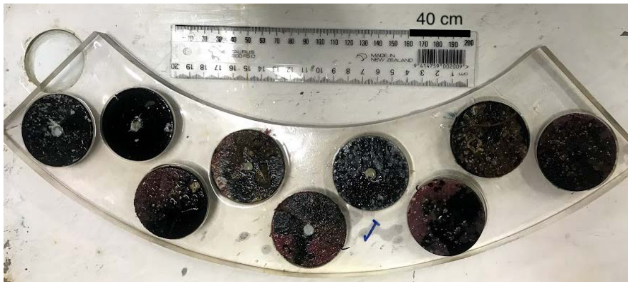
Figure 2.3 A quarter-circle acrylic insert used to create a false bottom in the annular flume during oxygen profiling. The nine slots, 5 cm in diameter and 1 cm thick, were filled with 5 cm discs, either covered with a mixed algal assemblage or empty.
