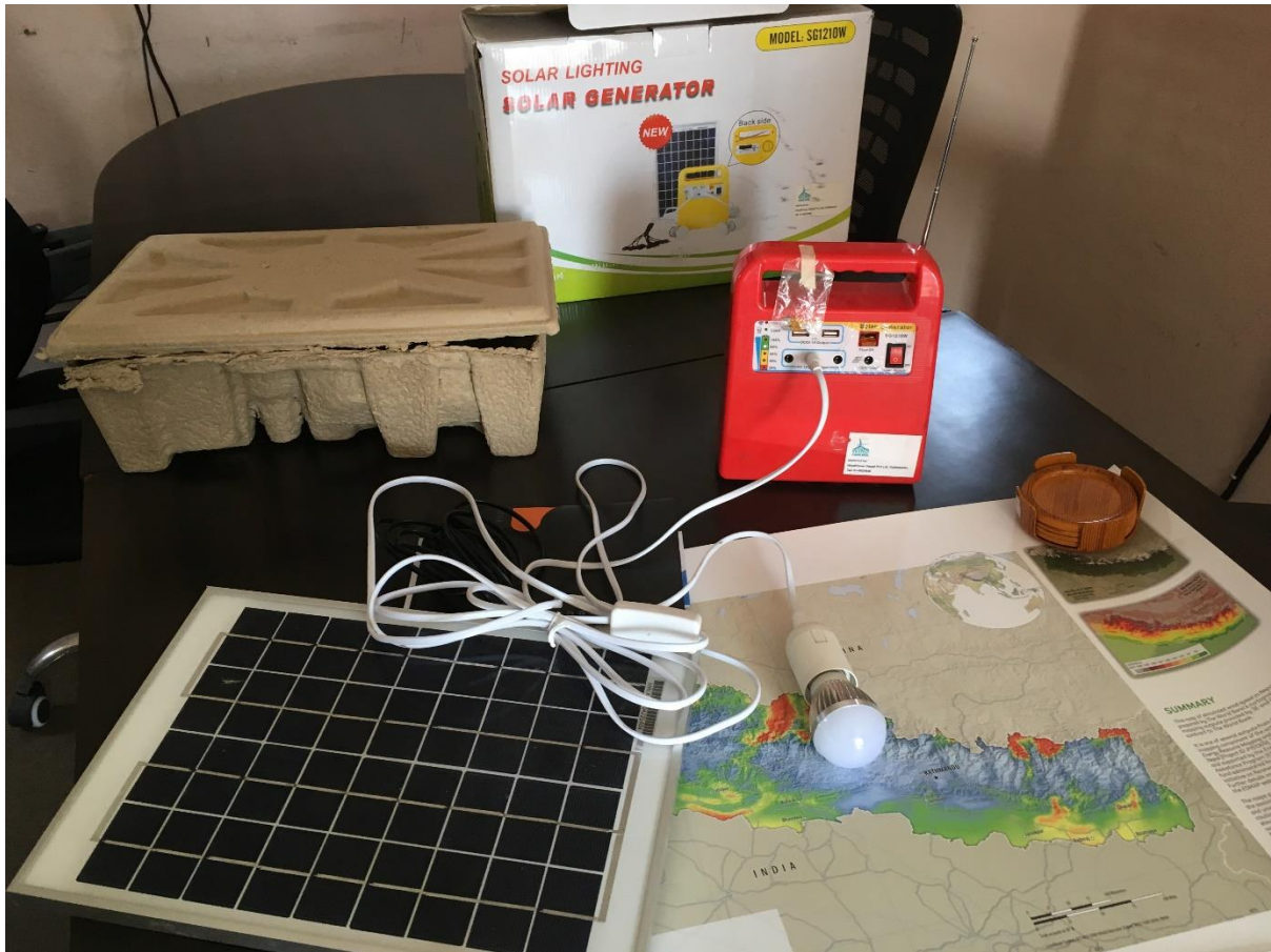
Figure 5.3.3: The small solar devices which were in high demand after the earthquake, due to their ability to provide light and cell phone charging without access to electricity system.
