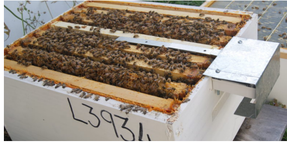
Figure 2.6: HiveMind colony strength monitor extending inside a hive. In the current experiment, the metal sheet extending into the hive was replaced by a cable with a temperature sensor at the end, extending to the same point in the hive. Image was sourced from https://hivemind.co.nz/ .
