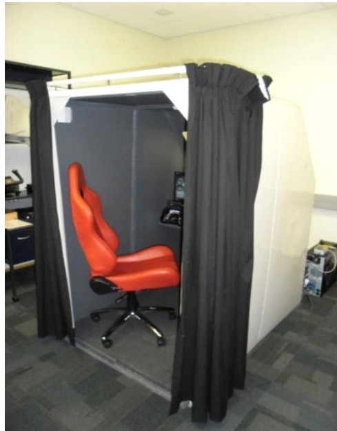
Figure 2. The flight simulator’s custom made fibreglass cabin. The cabin is facing a blank white wall where the external imagery is projected.
