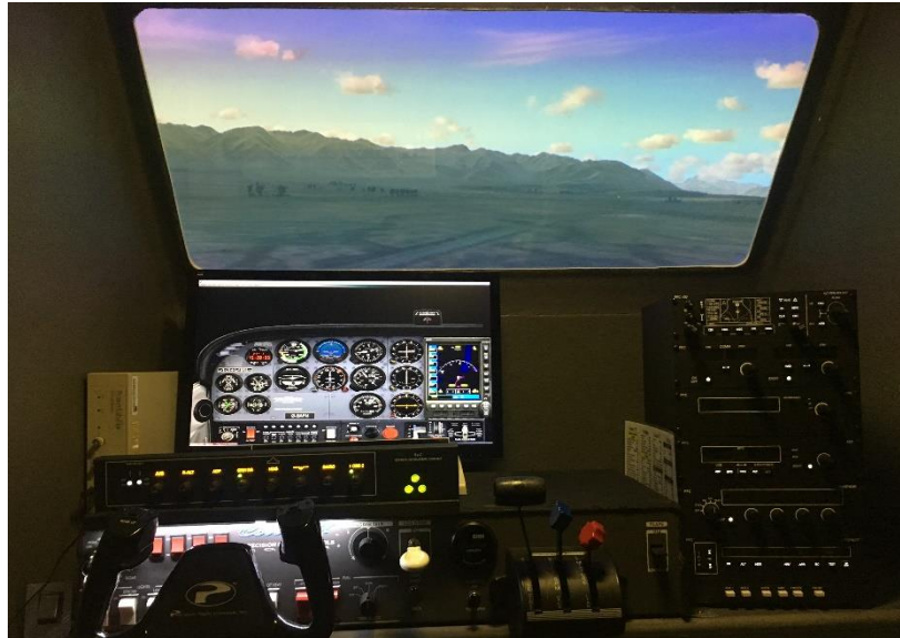
Figure 3. Flight simulator set up, a photo from inside the cockpit. The image includes the window and projected external image, the flight display (PFD and MFD) displayed on a LCD screen situated below the window, and the Cirrus II precision flight controls situated below the PFD. To the left of the LCD is a PowerLab running the ear mounted plethysmograph.
