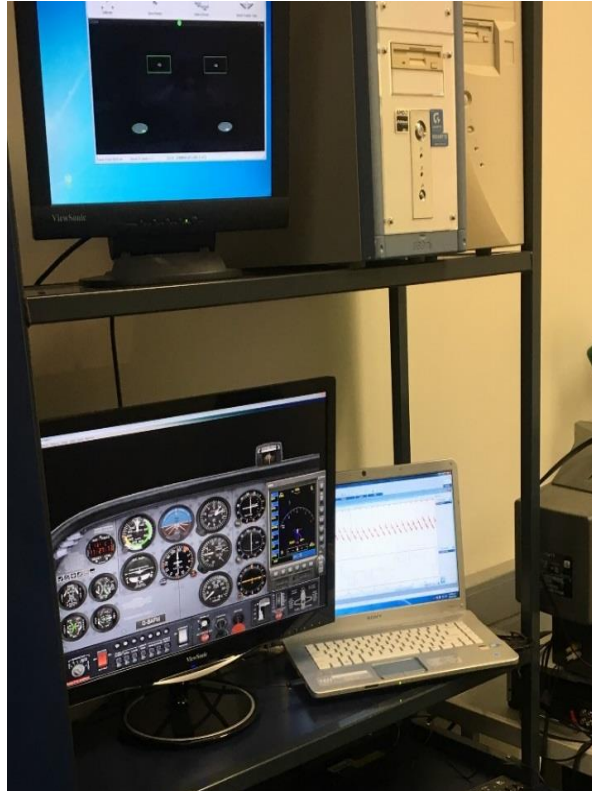
Figure 6. Picture of external control screens and laptop. The largest monitor is reflecting the screen inside the cockpit (displaying the PFD and the MFD) and allows for external experimenter control. The laptop runs the LabChart7 connected to the PowerLab and plethysmograph. The small top monitor shows the Gazepoint control screen.
