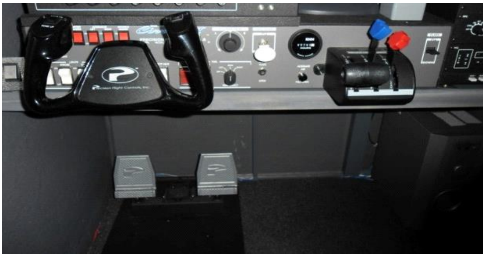
Figure 3. Flight simulator set up, a photo from inside the cockpit. The image includes the window and projected external image, the flight display (PFD and MFD) displayed on a LCD screen situated below the window, and the Cirrus II precision flight controls situated below the PFD. To the left of the LCD is a PowerLab running the ear mounted plethysmograph.
