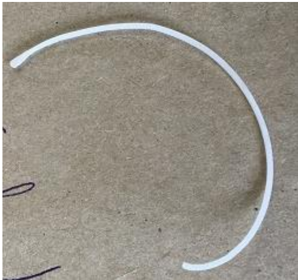
Figure 5: 1 PCL:PLA 30:70WT% plasticised with 20% PEG-200 2 pass variant. Permanent shape.
