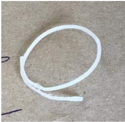
Figure 5: 3 PCL:PLA 30:70WT% plasticised with 20% PEG-200 2 pass variant. Deformed shape
