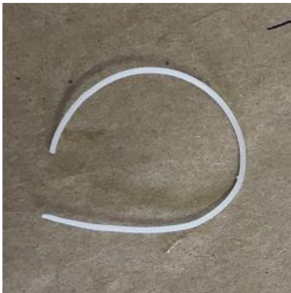
Figure 5: 2 PCL:PLA 30:70WT% plasticised with 20% PEG-200 2 pass variant. Thermal Contraction.
