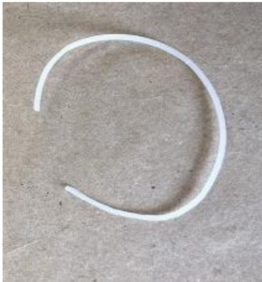
Figure 5: 4 PCL:PLA 30:70WT% plasticised with 20% PEG-200 2 pass variant. Recovered shape
