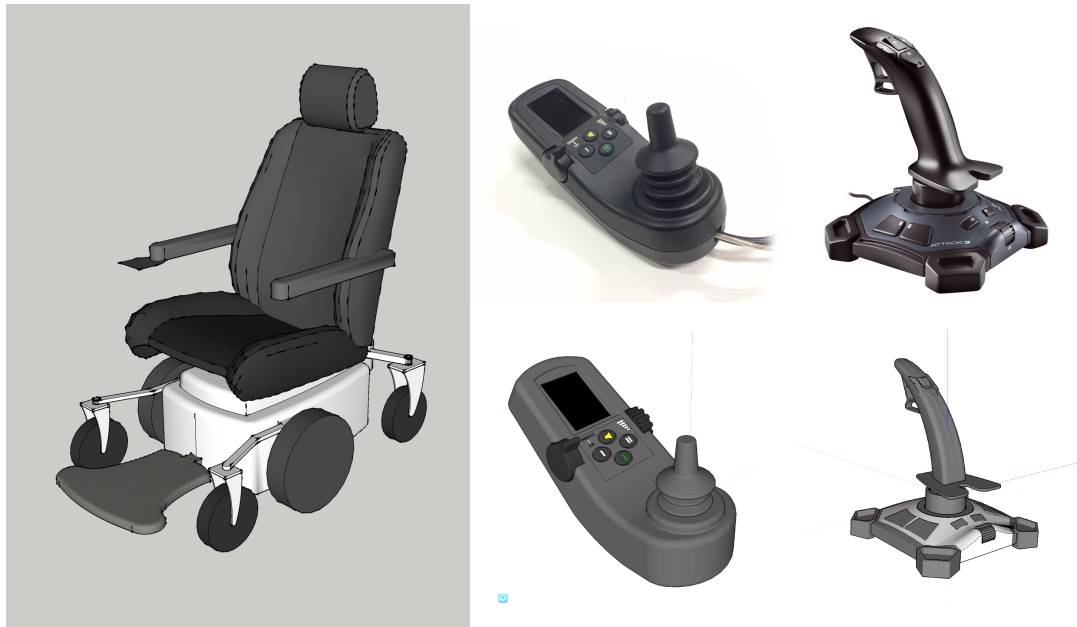
Figure 13: (Left picture) virtual PWC. (Right picture) real PWC and gaming joysticks (top), virtual PWC and gaming joysticks (bottom).
