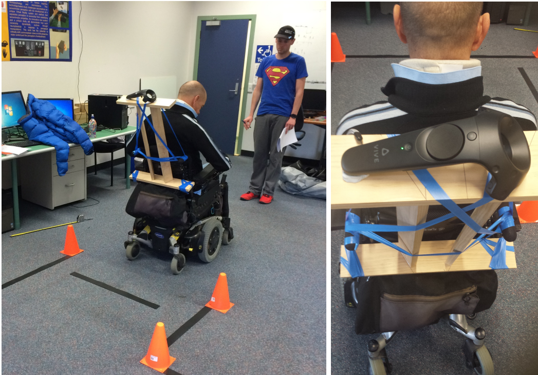
Figure 36: HTC controller placed on the wood frame to track the PWC movement
