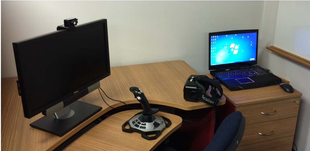
Figure 21: Experiment components, including monitor, joystick, HMD, laptop, and HMD tracker placed at the top of the screen
