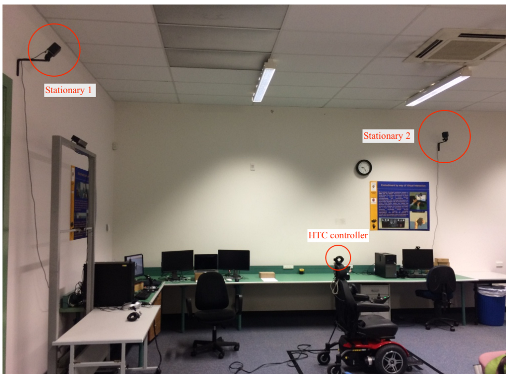
Figure 37: HTC base stations mounted on the walls and HTC controller placed on the PWC (This is not the actual PWC used for recording)
