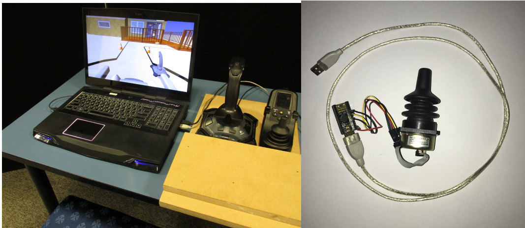
Figure 14: On the left, experiment setup: Alienware laptop and joysticks. On the right, Arduino board connected to the PWC joystick
