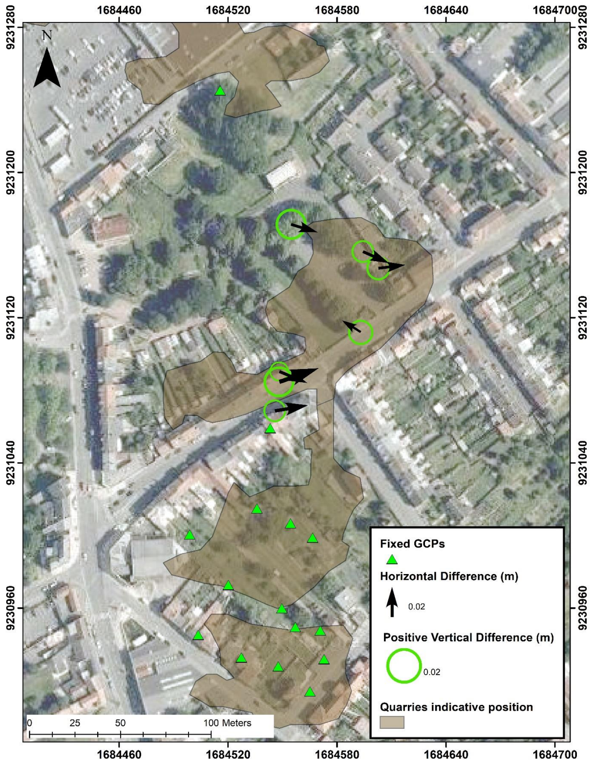
Figure 4.10. Scenario A3. Where no control was fixed in Wellington to replicate no control in the Auckland Quarry and areas outside the extents of the GCP control network.
