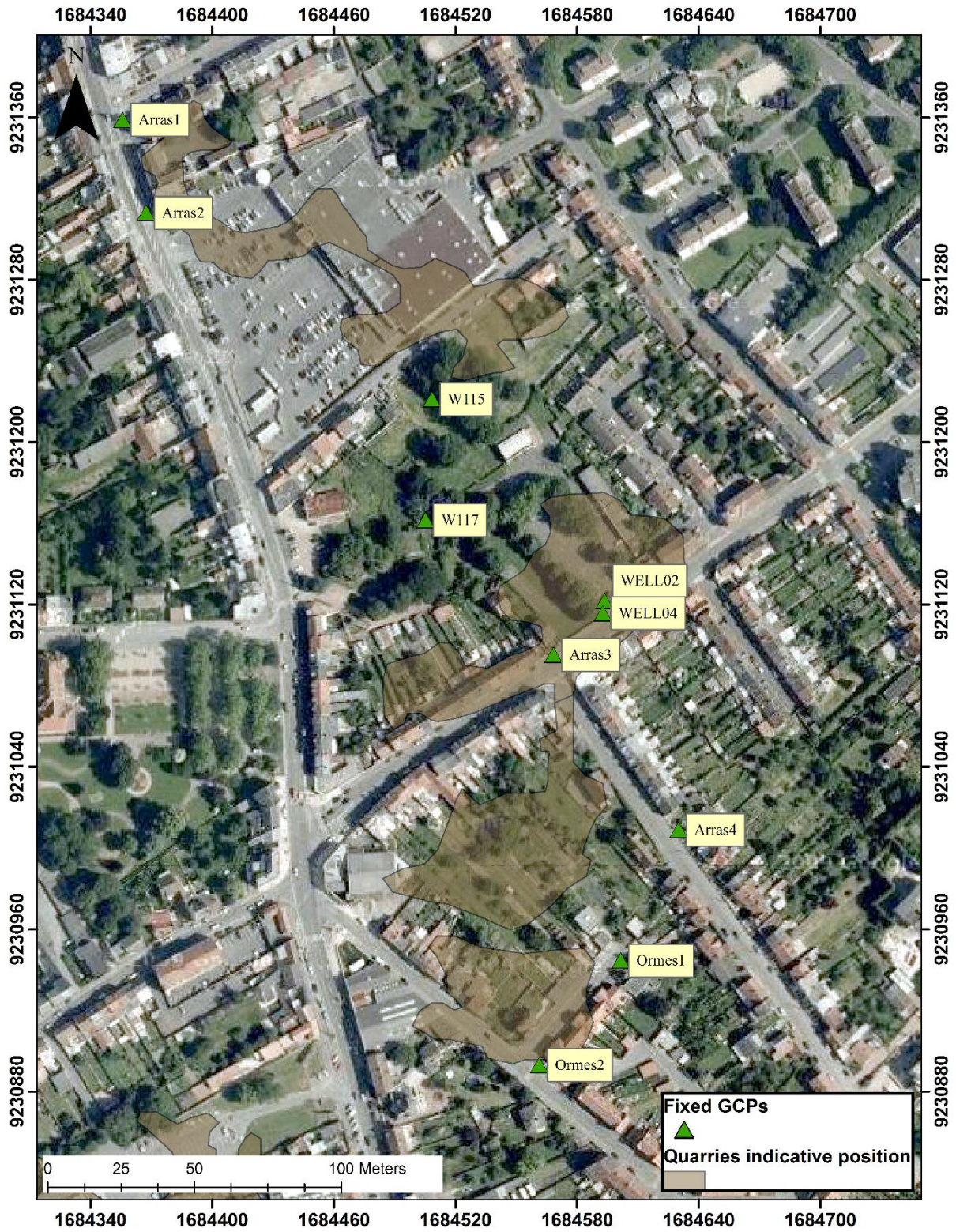
Figure 4.5. Ground control points used to georeference the streetscape.
