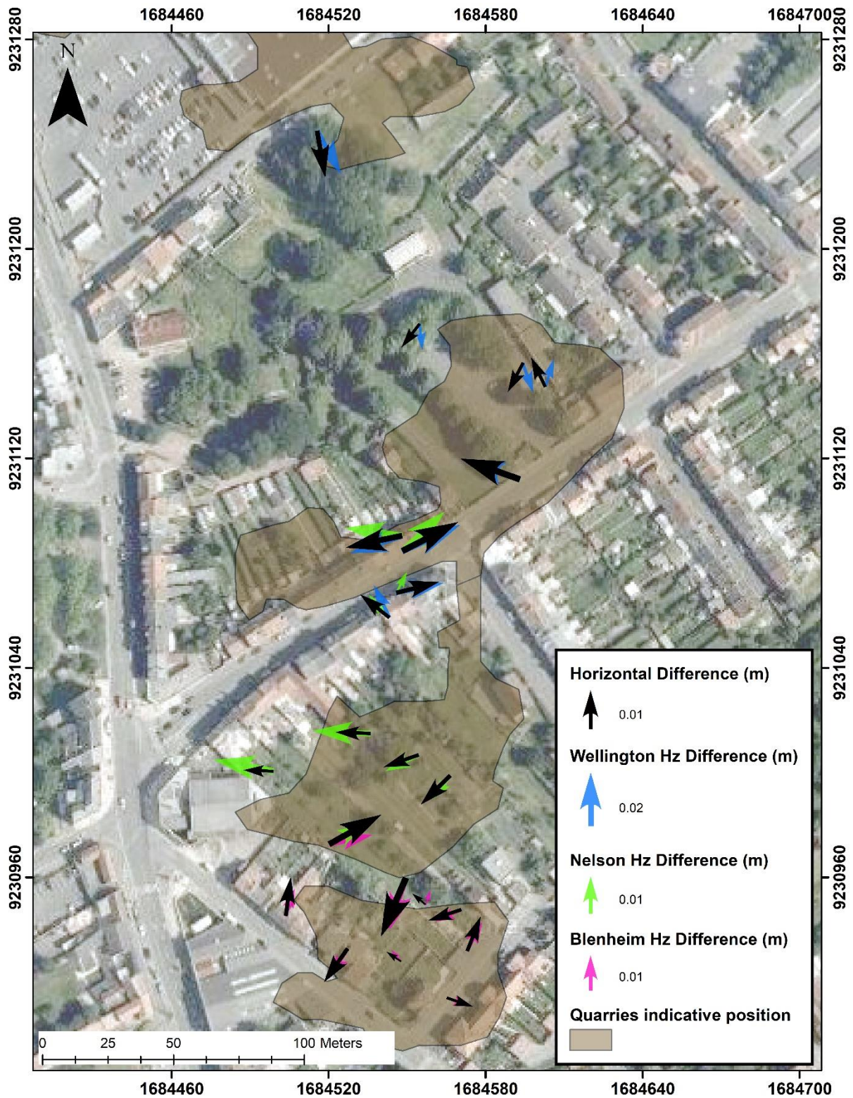
Figure 4.9. Scenario A2. A horizontal comparison between completing the georeferencing for the entire project point cloud against georeferencing each quarry individually.
