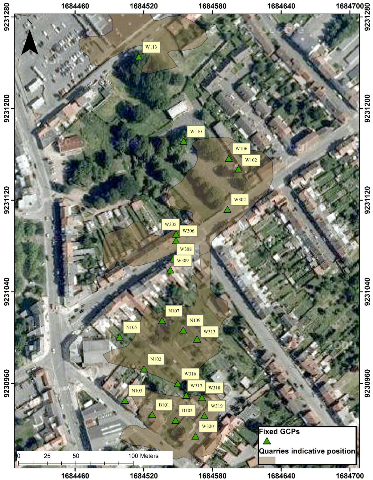
Figure 4.4. Ground control points used to georeference the underground quarries.
