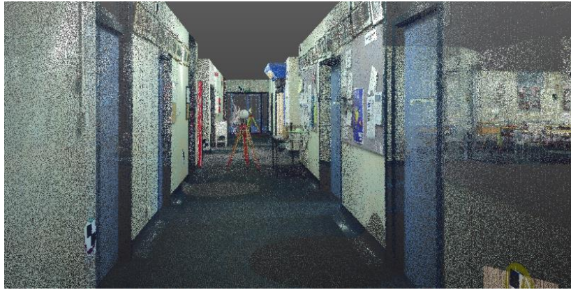
Figure 3.3. Point cloud data of scanned corridor, showing GCPs and CPs in the form of spheres and checkered targets.
