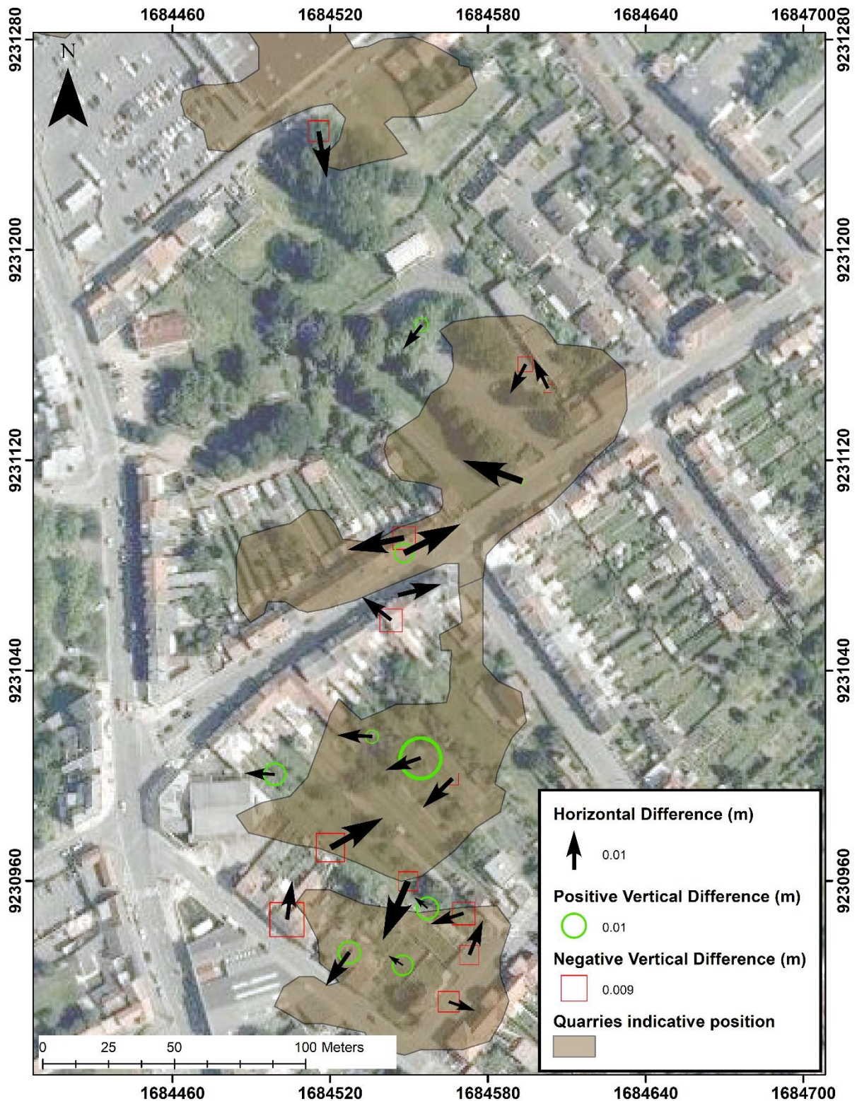
Figure 4.8. Scenario A1. Horizontal and vertical residuals between the total station and the TLS coordinates. The total station coordinates have been used as the known coordinates.
