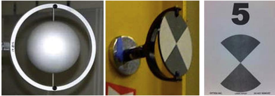
Figure 2.9. Target types used by Becerik-Gerber et al. (2011) for the investigation into various accuracies achievable using the above targets.
