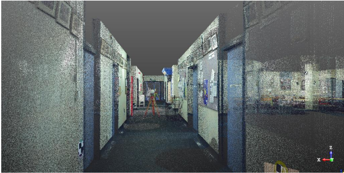
Figure 2.8. A typical example of common markers, showing checkered targets on the walls and a sphere on a tripod.
