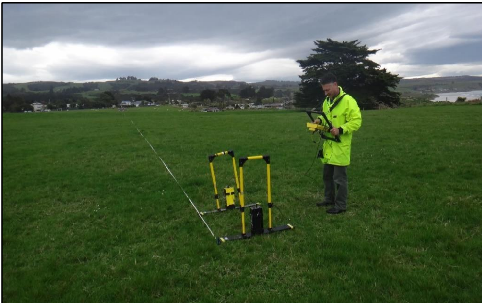
Fig. 3.10 The setup of our GPR survey. A 140 m long tape is laid out across the fault scarp and the paddles are placed 1 m apart.
