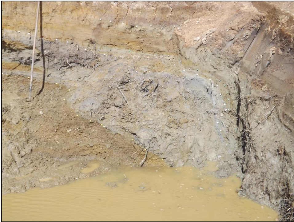
Fig. 2.13 The coloured nails mark the folding over of lithology on the southern wall of the Rocky Valley trench.
