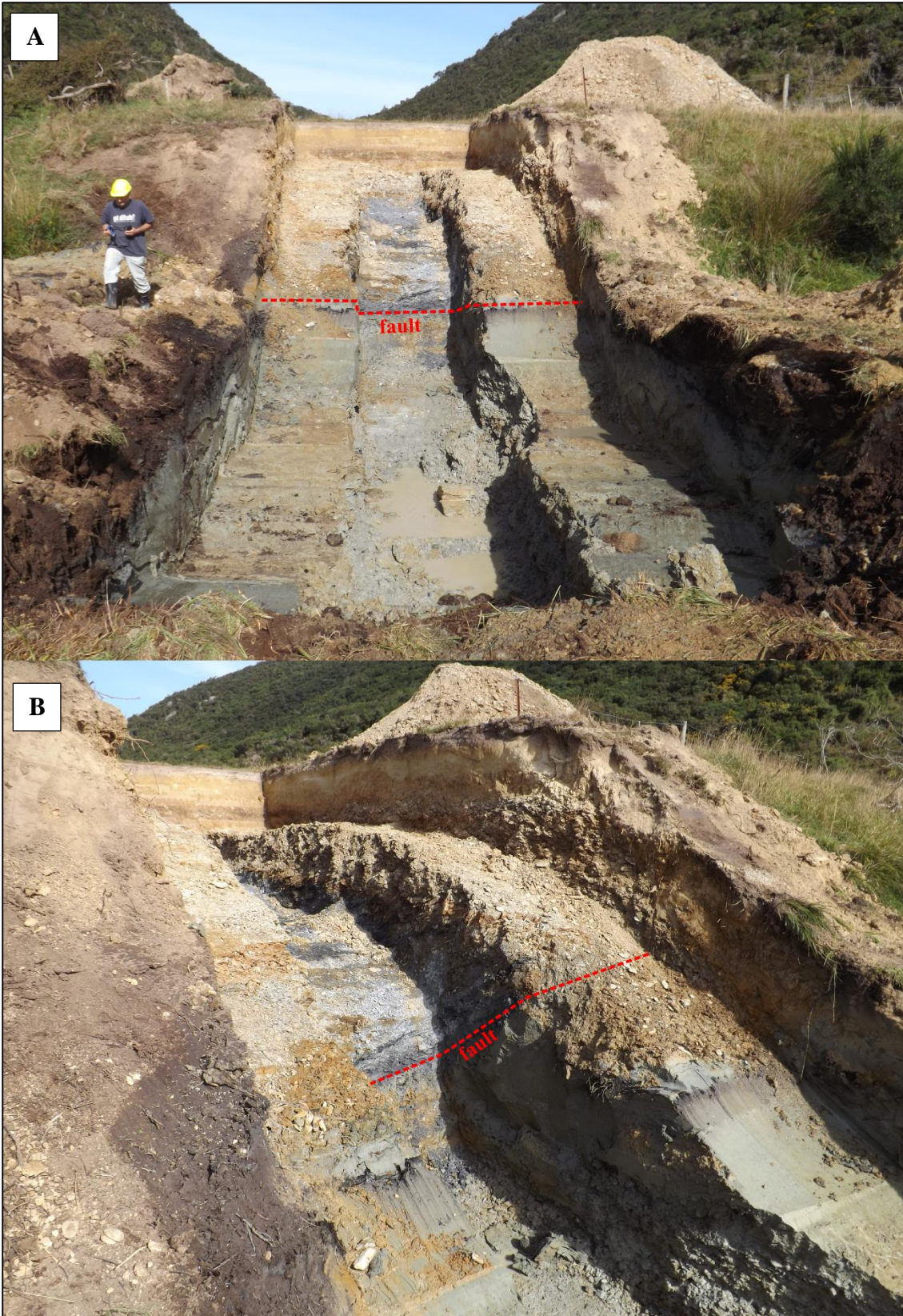
Fig. 2.10 Big Creek trench after excavation. The red dashed lines denote where the trench intercepts the Akatore Fault. A. View of the trench looking east, perpendicular to the scarp. B. The Akatore Fault on the south wall of the trench.
