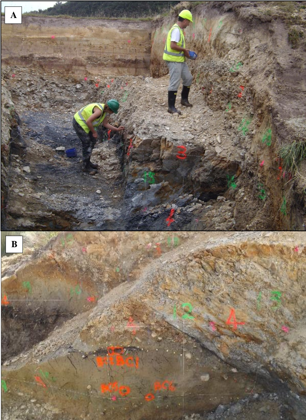
Fig. 2.11 Big Creek trench divided into 1 x 1 m quadrants with important features highlighted. A. The different lithologies with coloured nails are being marked on the south wall in the image. B. View of the Akatore Fault (schist overlying sediments) on the north wall. Writing in orange corresponds to radiocarbon sample locations.
