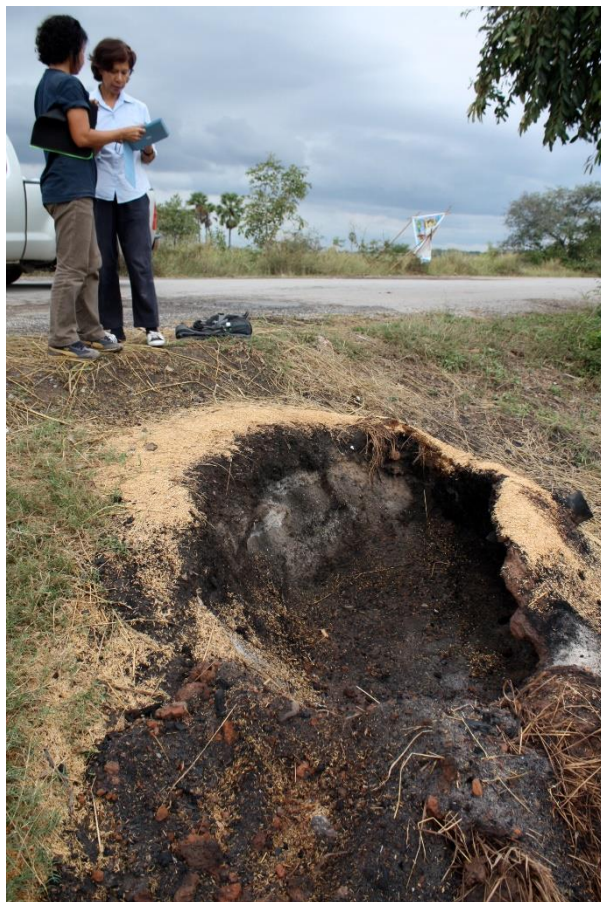
Figure 3-2 Charcoal kiln that has been deconstructed to collect the charcoal, note the can in the right of the structure which was used for airflow and the covering of rice chaff for insulation, photo courtesy of Charles Higham.
