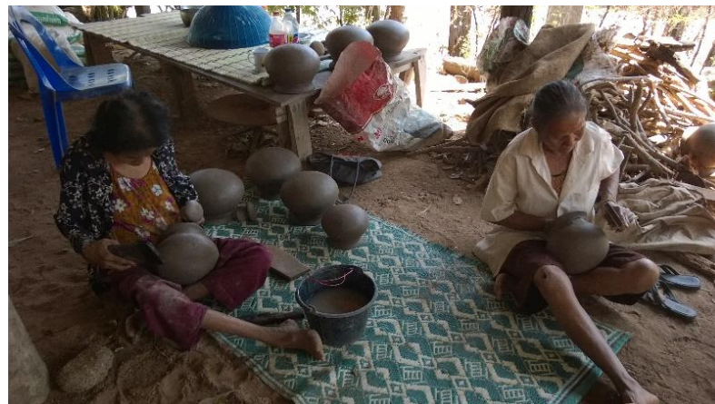
Figure 5-8 The sisters Eyang and Yai forming the bodies of the vessels.
