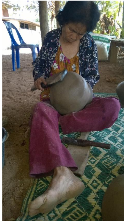
Figure 5-7 Forming the base and the shape of the body.
