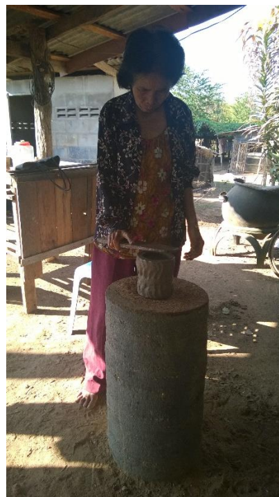
Figure 5-4 Flattening the preform.
