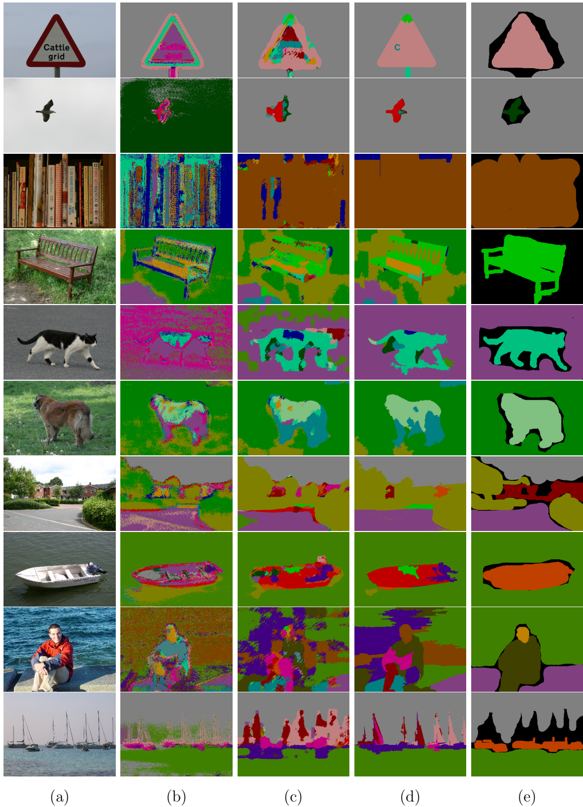
Figure 7.4: Semantic segmentation from different random forests: (a) the original, (b) standard random forest, (c) structured random forests, (d) structured random forest with unsupervised segmentation, (e) the ground truth with class labels shown in colour (the void label is in black).
