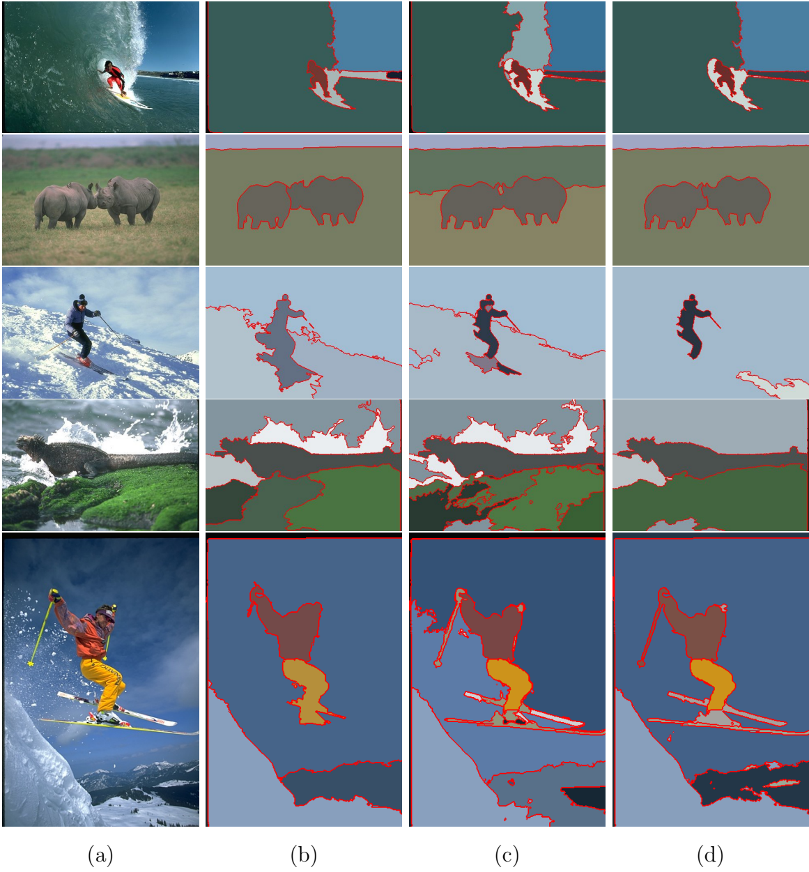
Figure 6.6: Segmentations from different approach: (a) the original (b) SAS (c) CCM (d) SHST*. SHST* tends to partition the image with fewer segments.
