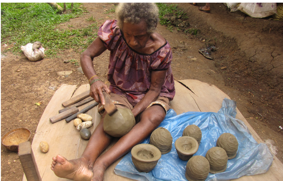
Yeyeg beating the body of the pot into shape using a wooden paddle.
