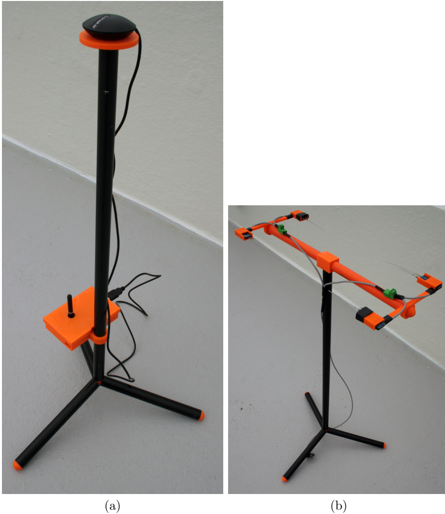
Figure 3.3: Figure (a) shows the stand for the GlobalSat BU-353S4 GPS unit with the higher-quality aerial. The base is magnetised and a steel bolt threaded in the stand allows it to stay securely mounted. The case seen at the bottom of the stand contains a Raspberry Pi for data collection and storage. The aerial seen on the case is from a board attached to the Pi to receive telemetry signals from the tag style units. Figure (b) shows the set of 4 tag style GPS units developed by the Electronics Research Group at the University of Otago.
