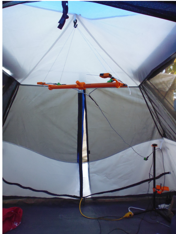
Figure 3.7: Unfortunately the stand for the four tag-style GPS units broke while on North Stradbroke Island. In order to be able to store the equipment required and not risk accidental damage to the tags it was decided to suspend them as shown.
