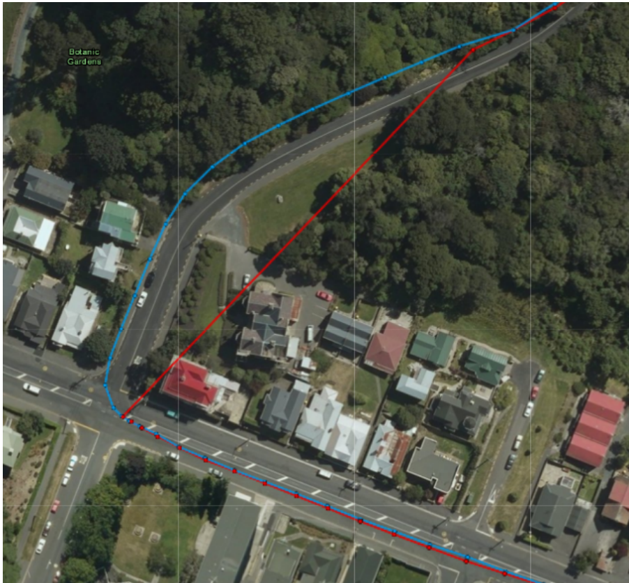
Figure 1.3: The red waypoints are the GPS signal that the combined navigation system was using. We simulated a loss of GPS signal by removing fifteen seconds of GPS data to see how the system would cope. The blue waypoints are the estimated position from the combined system.
