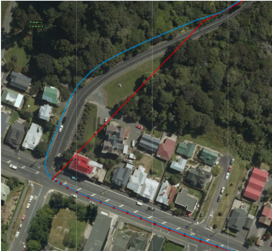
Figure 7.17: The same fifteen second simulated GPS signal loss but with an integrated GPS and IMU system. The combined system with the simulated signal loss is the blue path while the red path is the original GPS signal.
