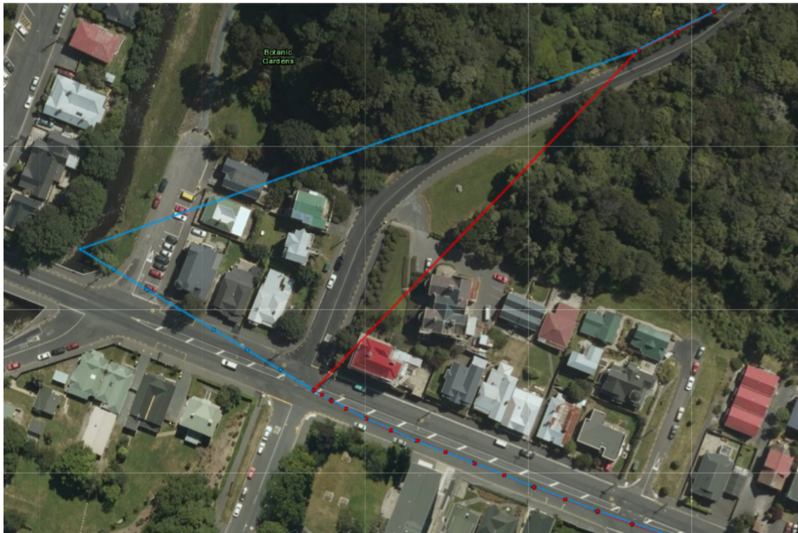
Figure 7.16: A fifteen second loss of GPS signal was simulated. The blue track shows the results from a solely GPS-based navigation system, operating on the assumption of a constant speed and heading between samples. The red track is the GPS signal with the fifteen seconds of data removed.
