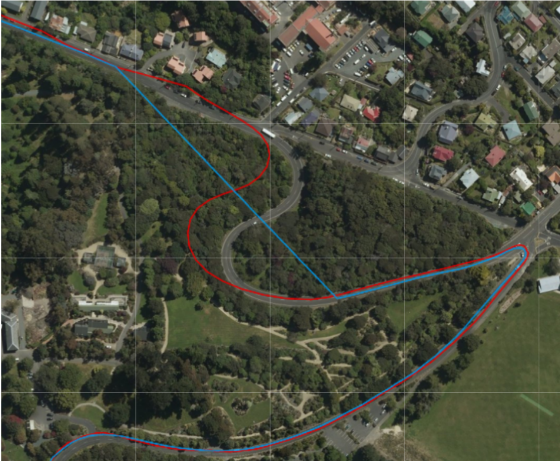
Figure 7.21: When undergoing hard cornering or large accelerations the filter has some difficulty correcting quickly enough. As seen during this 30 second interval.
