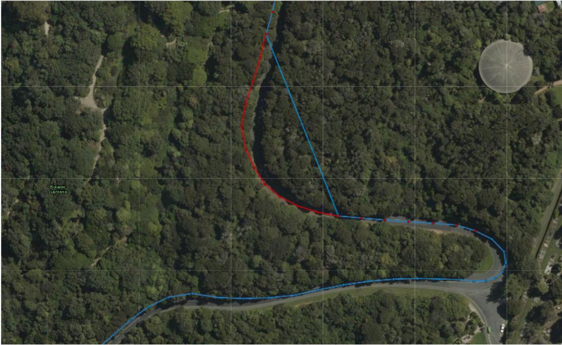
Figure 7.19: The effects of losing signal at another corner. Again the GPS measurements used by the filter are plotted in blue, while the filter output is plotted in red.
