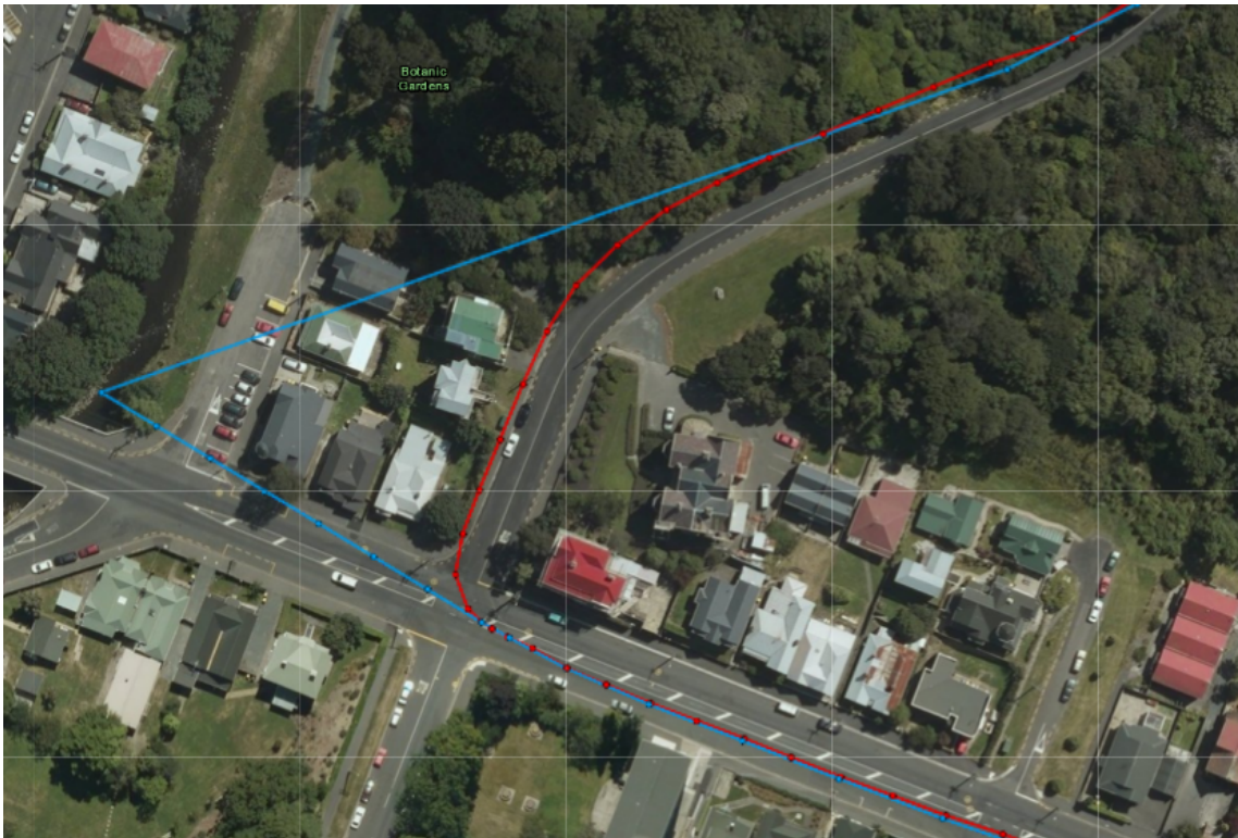
Figure 7.18: Both sets of data here had the same fifteen second period of GPS measurements removed to simulate a loss of GPS signal. The track in blue shows the results of such a loss of signal on a GPS-only navigational system while the track in red shows the results of such a loss of signal on a combined GPS and IMU navigational system.
