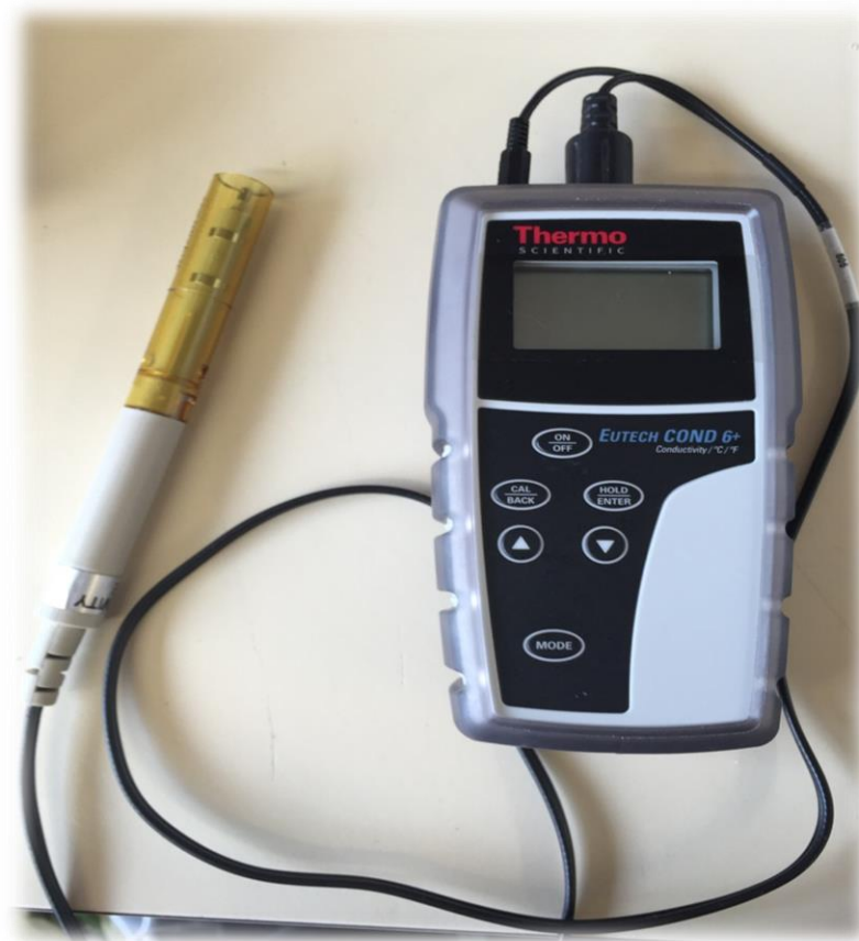
Figure 14. Conductivity meter, the two-terminal electrode and the plastic cover guard.
