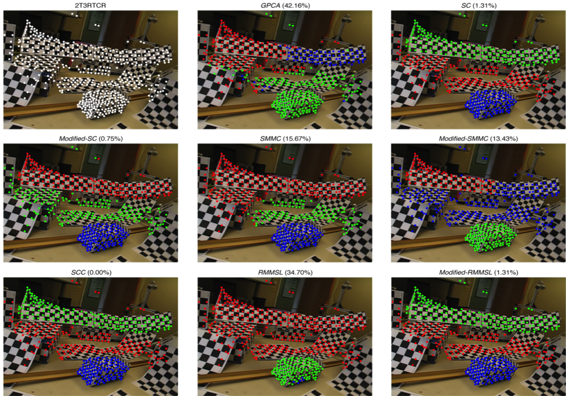
Fig. 3.9. Clustering results for 2T3RTCR video sequence. There are 26 frames in this data set. The camera is rotating in the video, and the long checkerboard in the middle is swaying.
