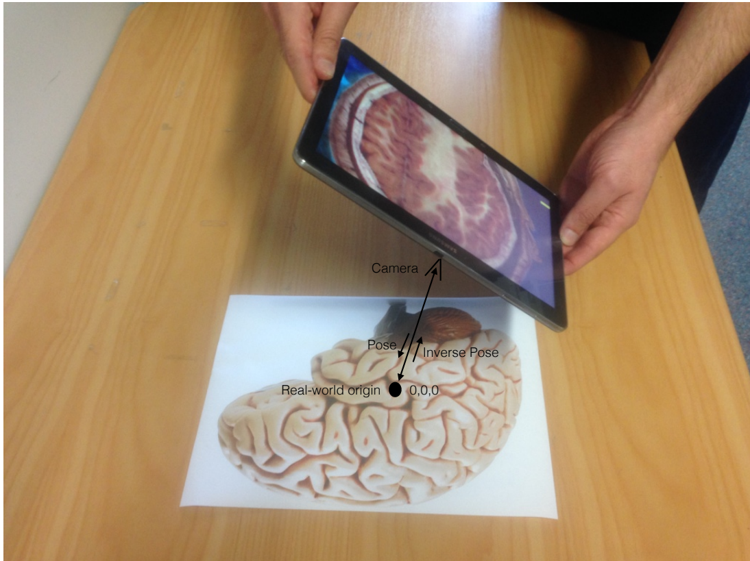
Figure 5.3: Our starting scene that consists of our tablet camera and visual marker which defines our real-world origin at the center of the visual marker
