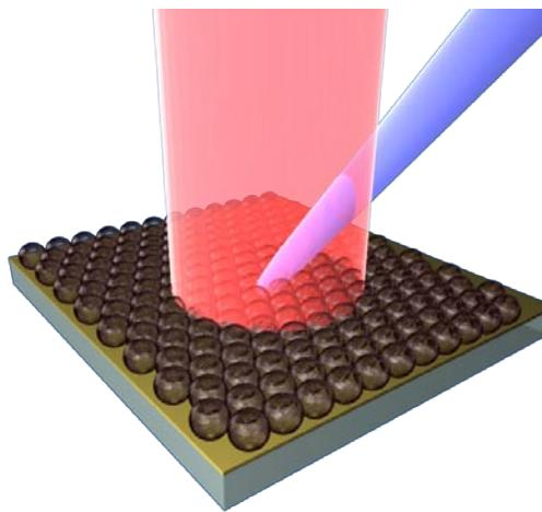
$\Phi = 520 \text{ nm}$  Red Dye doped PS spheres pumped
