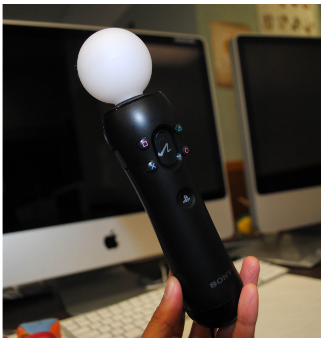
Figure 4.4: PS Move’s motion controller with a sphere attached for tracking.
