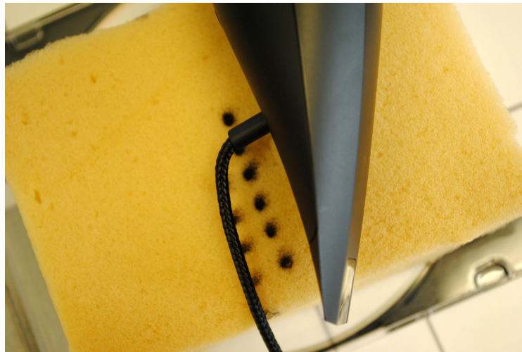
Figure 5.1: To find the center of rotation, the wire that sticks out from the controller's tail is placed on one of the dots to mark the possible position of its center.
