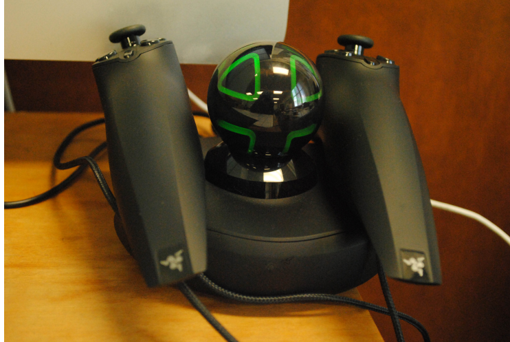
Figure 4.6: The Razer Hydra - consists of a base station and two motion sensing controllers.
