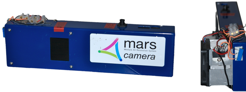
Figure 6.1: The MARS camera with quad Medipix3 detector and fan-assisted Peltier cooling system.
