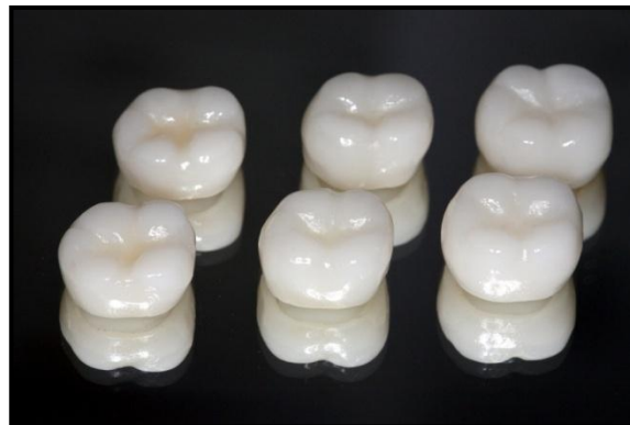
Figure 3-14: 1mm, 2mm and 3mm cusped zirconia crown samples from left to right
