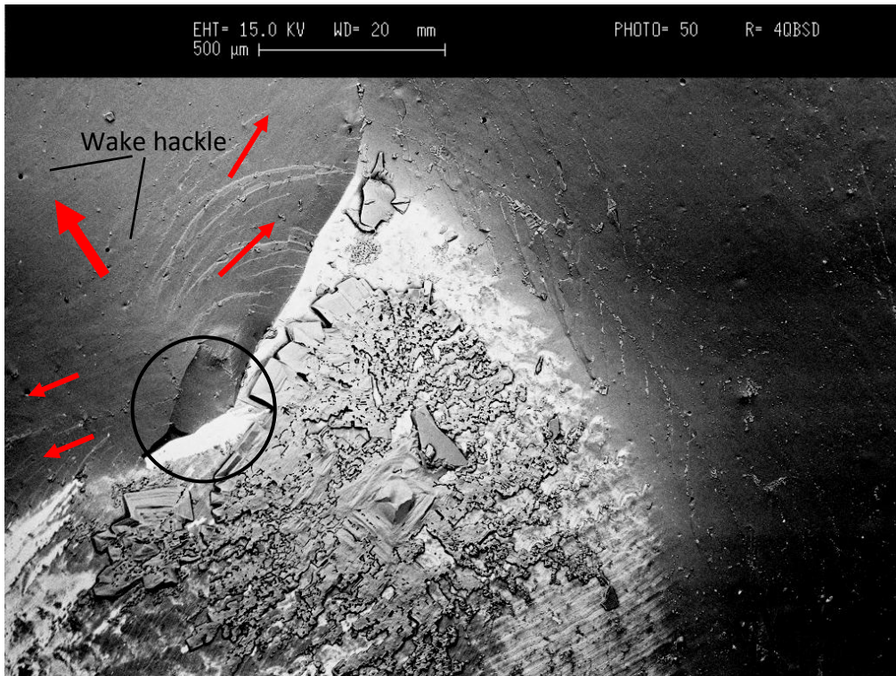
Figure 4-45: SA1 - Back scatter detector image of delamination zone shows primary origin of fracture at the base of veneering porcelain (black circle) [magnification x 50]
