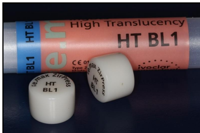
Figure 3-10: Sample of IPS e.max ZirPress ingots used in this study
