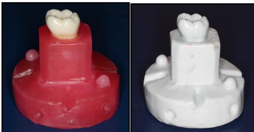
Figure 3-2: Model tooth in waxed jig (left), epoxy resin duplicate of jig (right)
