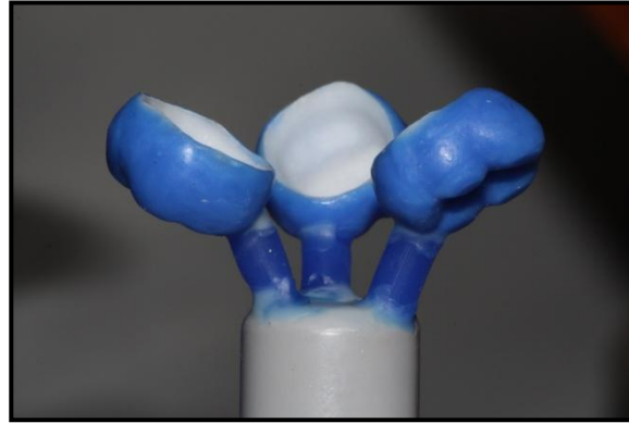
Figure 3-11: Three waxed zirconia copings sprued and ready for investment
