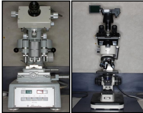
Figure 3-16: Vickers indentation machine (left); optical light microscope with digital camera fixed to the top viewer (right)
