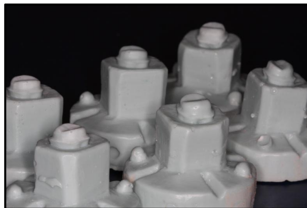
Figure 4-3: Prepared epoxy resin abutments ready for sample cementations
