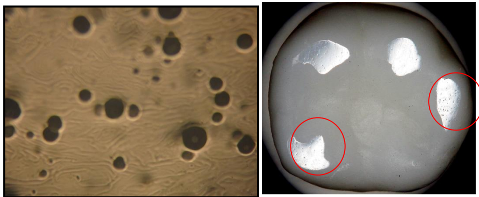
Figure 3-9: Porosities found on the surface of zirconia copings pressed with IPS e.max ZirPress, light microscopic view (left), porosity can also be seen without magnification (right)
