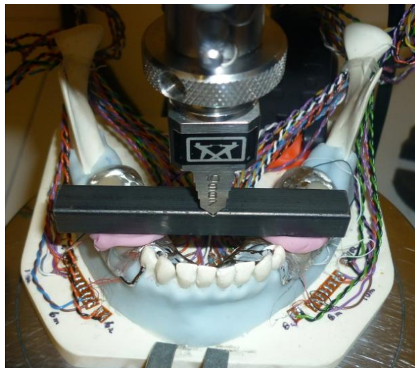
Figure 12: Bilateral loading of premolar region in Instron universal testing machine
