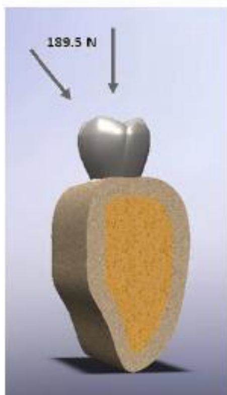
Fig. 3 Implant-bone model under loading force of 189.5 N
