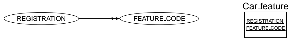
Figure E.2: Translating a multivalued dependency to and from a Martin ERD (rule S2)
