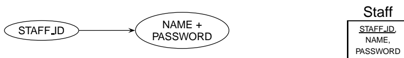
Figure E.1: Translating a single-valued dependency to and from a Martin ERD (rule S1)
