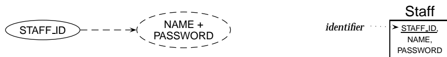
Figure E.3: Translating a single-key bubble between an FDD and an ERD (rule S3)
