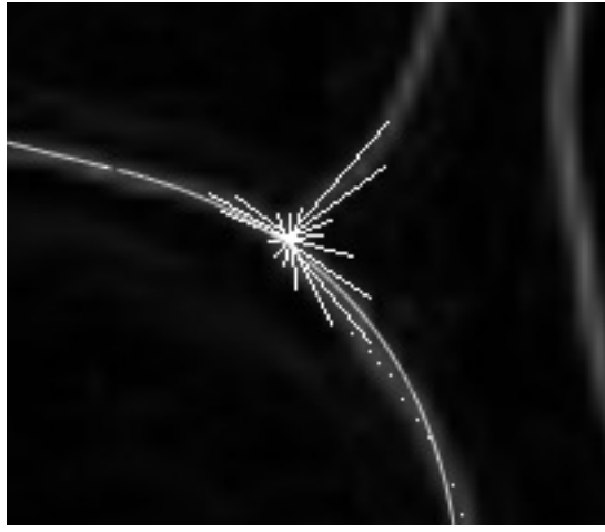
Figure 2: Visualisation of the evaluated direction vectors. The length of the vector indicates the average gradient in that direction.
