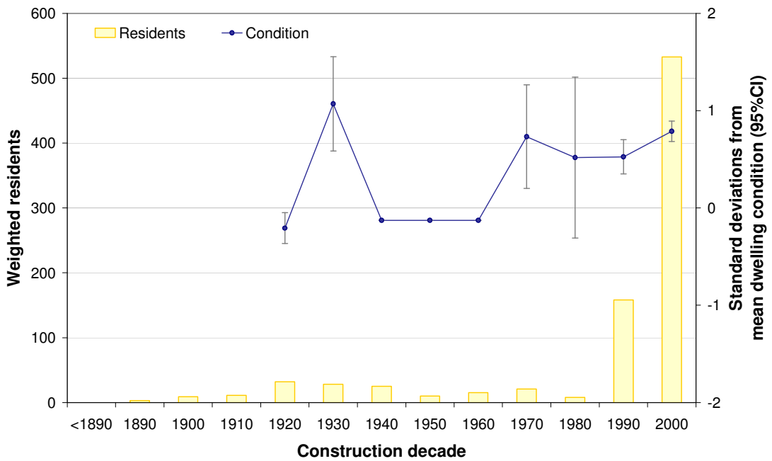
Figure 6.47 Number of Apartment residents (weighted by study person days); and standard deviations from mean dwelling condition for all dwellings, by decade of Apartment construction (Matched QV/NHI data).
