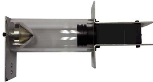
Figure 3: Catadioptric system design and assembly using a transparent extruded thermoplastic acrylic tube.
