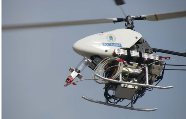
Figure 1: UPM-COLIBRI III Electric Helicopter platform during an Omnidirectional attitude and heading estimation tests using a catadioptric camera
