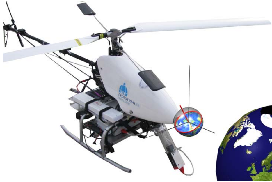
Figure 4: Skyline is the occluding contour of the earth sphere surface, whose projection on the equivalent unitary sphere model through a plane that intersect it forms the depicted red circle.
