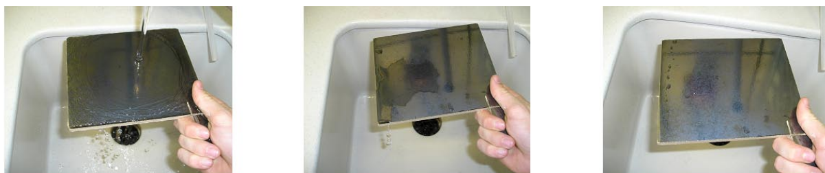
Figure 4. Test in which the tile with a metallised appearance displays hydrophobicity.
