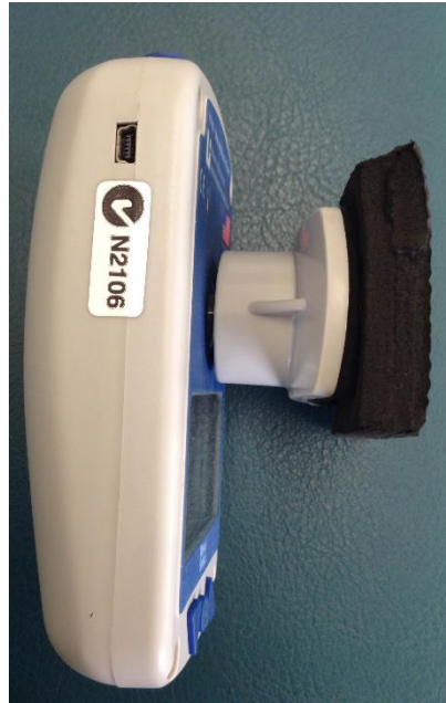
Figure 5.1. Lafayette device used for strength and power assessment with additional foam padding attached.
