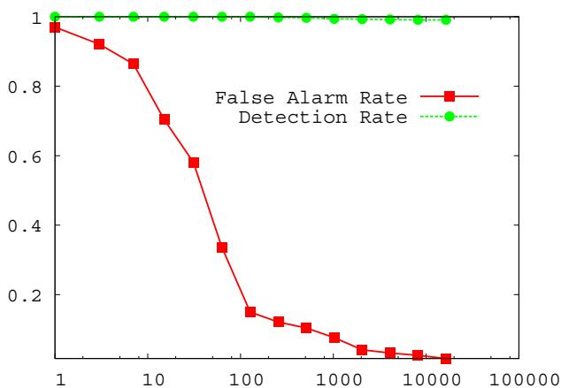
Figure 5 (b). The false alarm rate and the detection rate vs the number of training requests is plotted
