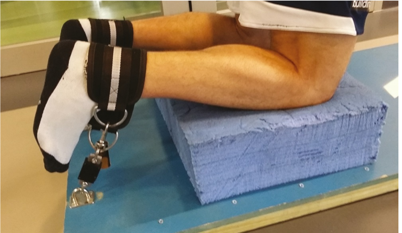
Figure 3-2. Close up of the ankle brace and in-series, uniaxial load cells which determine eccentric force during the Nordic hamstring exercise.
