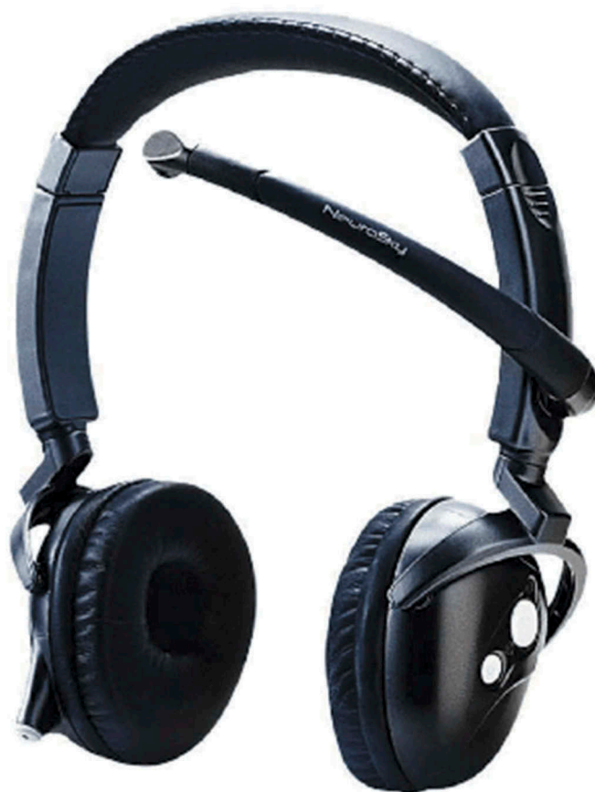
Figure 1. The NeuroSky mind-set consists of a single electrode embedded in a flexible arm extending from the left side of a pair of headphones (Image available via Creative Commons License BY-NC-SA 4.0).
