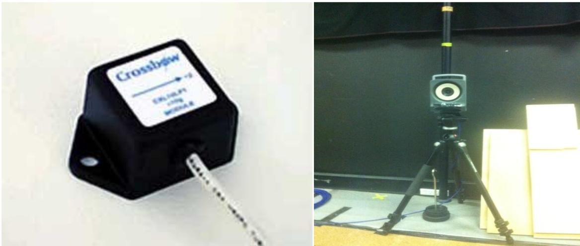
Figure 3.2. A tri-axial accelerometer (CXL25GP3, Crossbow Technology, San Jose, USA) and a 3D motion analysis camera (VICON Oxford Metrics, Oxford UK). The images are not to scale.
