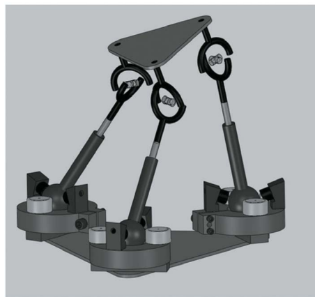
Fig. 4 Underactuated manipulator with topology 3-nSPU: (a) kinematic model, (b) 3D CAD model of a manufacturing scheme
