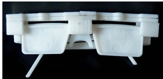
Fig. 10 Front view of the spectacle lens prototype using fused deposition modeling.
